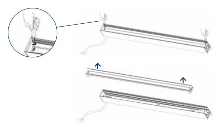
3 Continue with the rest of the luminaires. The end unit shall have one cover plate, one end cap and the power cable removed. Middle units shall have both cover plates, both end caps and the power cable removed.
