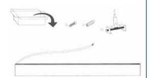
2 Fasten the mounting stud to the ceiling.
