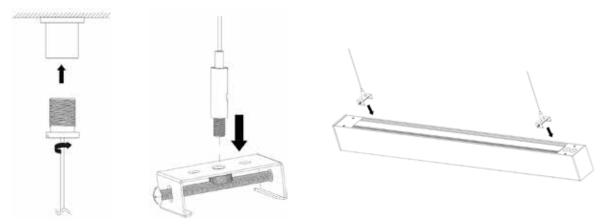
4 Adjust the luminaire's height so that its bottom is positioned 2 meters above the floor level. Cut suspension wire to appropriate length, leaving room for future adjustments. Tuck in the remaining wire neatly underneath the bracket. Remaining wire can be placed in the slots next to the top side light source.
