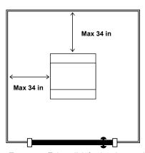
To get a sufficient disinfection dosage the <u>recommended maximum</u> distance from wall to UVEN unit is 34 in.
