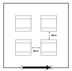
To get a homogeneous disinfection distribution the recommended distance between UVEN units is 48 in.
