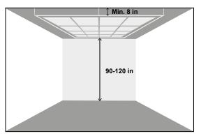
A supporting structure where the minimum height between ceiling grid system and inner ceiling is 8 in. Ceiling height between 90 and 120 in, measured from floor to suspended ceiling.
