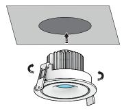
**4.)** Twist and tilt the luminaire to light up the desired area. See product specification for possible angles.
