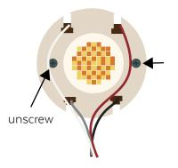
If re-placing the light source (LED COB) use thermal paste between the lightsource and heat sink and remount the luminaire by following this instruction in reverse.
